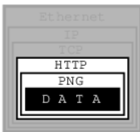
Figure 2. Sockets Covered Protocol Layers
